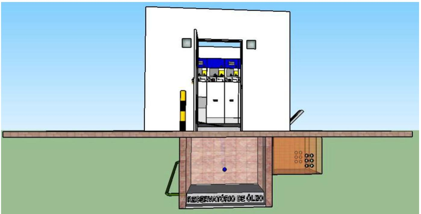
**Anexo XI - Estação transformadora abrigada e câmara de manobra****Figura 45 - Estação Transformadora para 1 transformador de até 225 kVA (9/9)**
